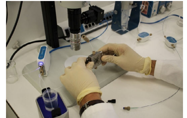
Figure 4: Holding the RayDROP to evacuate the air
