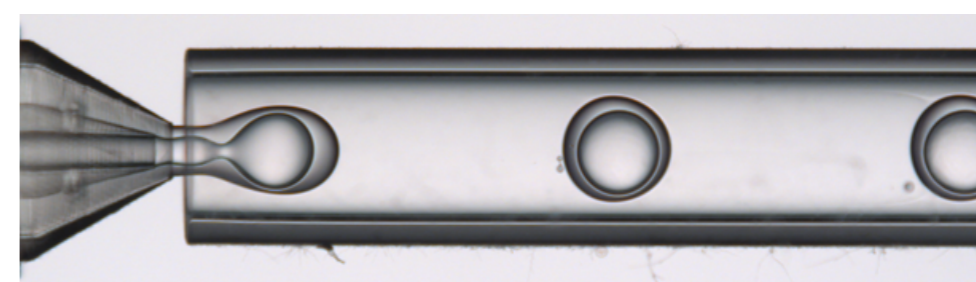
Figure 8: Generation of droplets in the Raydrop®.
