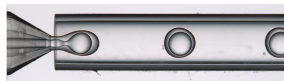
Figure 8: Generation of droplets in the Raydrop®.
