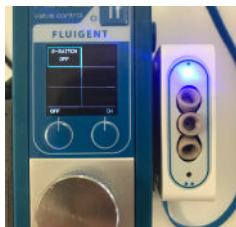
2-SWITCH™ in position 1
