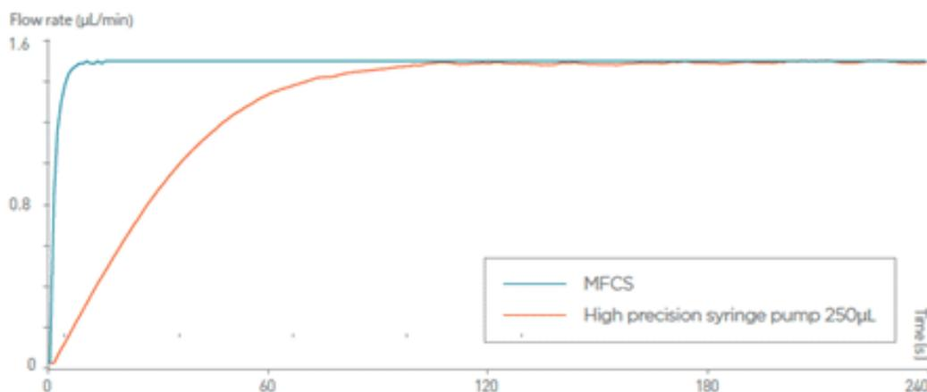
**FLUIGENT** Technology allows to obtain a fast flow rate response over the time . With a **short settling time** and **quick pressurization of systems**. Compared to syringe pumps, **MFCSTM-EZ** allows to save experimental time, precious samples and expensive reagents with significantly **shorter response times compared to syringe pumps**.
